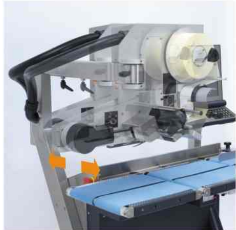
Label placement by lateral printer adjustment
