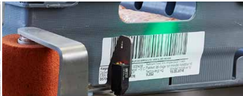
Automatic quality control of the label
