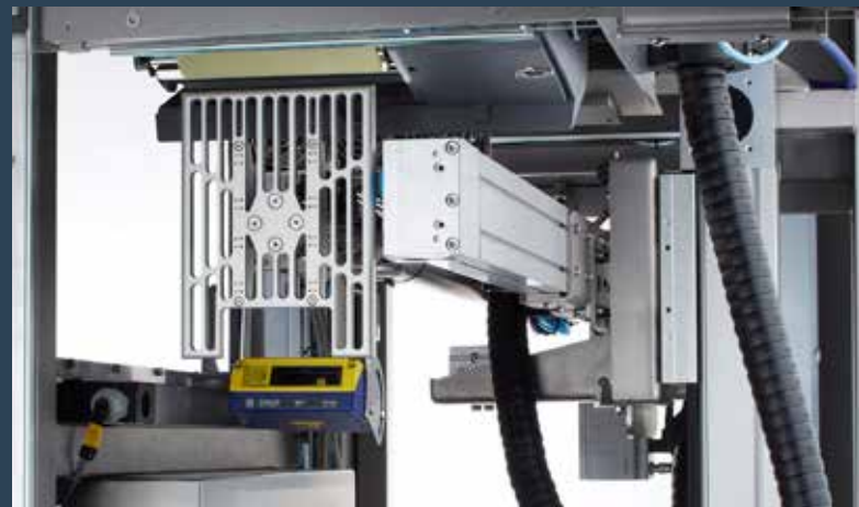
The servo motor ensures fast and accurate label application
