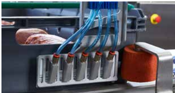
Automatic height adjustment of label application
