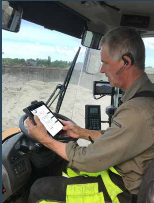
The ScanLoader module enables the operator to register the weight of the material he loads on to the lorry on his tablet or smartphone.
