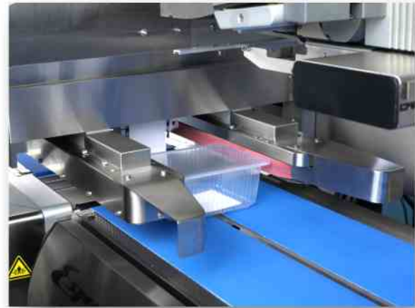
The package is guided precisely by the lateral guidings.
