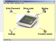
To use them, one of the 'function variants' in the instrument is activated. This puts DISOMAT into a configuration for specific applications that both allocates the essential actions to the six function keys and assigns the inputs and outputs of the instrument to the matching signals.
