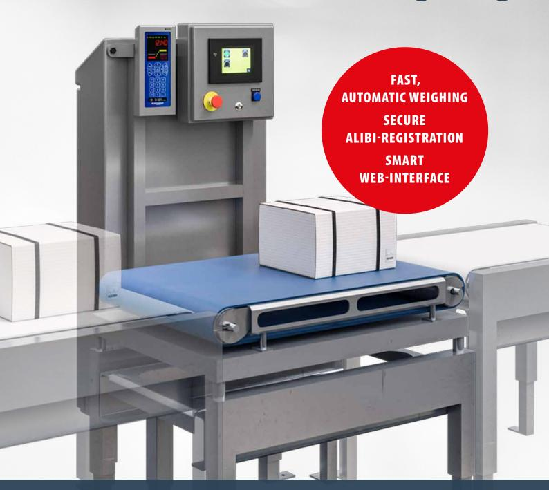
Scanvaegt Box Weigher is a complete system for automatic weighing of boxes and bulk products and registration of associated alibi-numbers.
