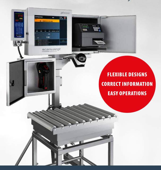
This ScanPlant NG module delivers flexible label designs and - combined with system integration - ensures correct information printed on the labels. This makes working procedures more effective and reduces the number of errors.
