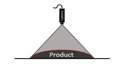
The PORTIO 3 uses the same top camera in combination with 2 cameras from the side. This allows scanning the contour of more rounded products, to prevent blind spots on the edges. Typical products are meat, sausages or whole fish.
