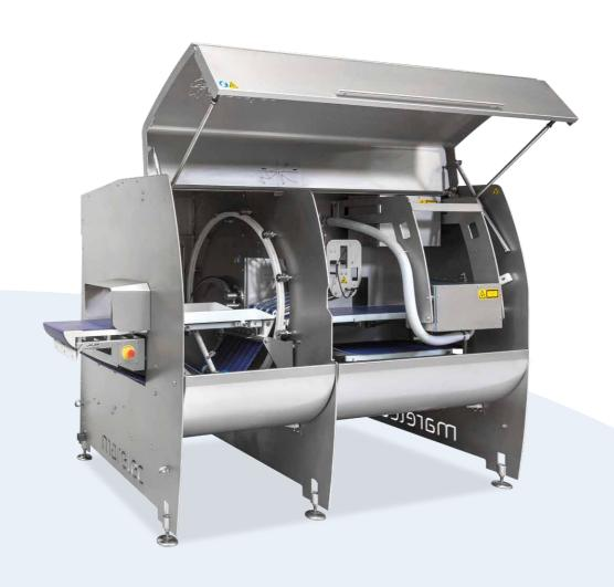
A PORTIO 3 adds two lateral cameras to the PORTIO 1. This allows the machine to improve the scanning and cover blind spots at the side of the product that cannot be detected by the top camera only. It is used for accurate portioning red meat or whole fish or any product with an irregular shape, in a vertical way. The machine can be equipped with the options mentioned on page 20.
