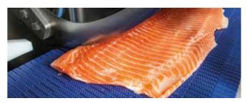
With a cutting rate of up to 25 cuts per second the ScanCut 1DAP delivers the highest capacity on cutting poultry products and smaller fish fillets. The portion cutter with dual lanes and 229 mm wide belts allows the processing of products with a width of up to 210 mm.
