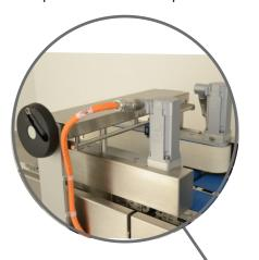
As the Powered Side Drives prevent the pack from slipping, the label placement will be accurate. The powered Side Drives and Signature labeller ensures the perfect label placement every time.
