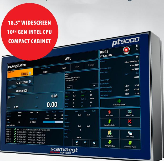
The Scanvaegt pt9000 mk4 is a high-speed, powerful and user-friendly industrial computer with an 18.5" touch screen for handling tasks like production management, order packing, dispatch, data collection and monitoring.
