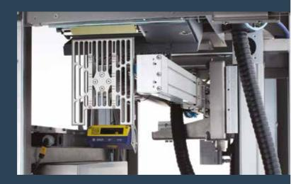
The servo motor ensures fast and accurate label application
