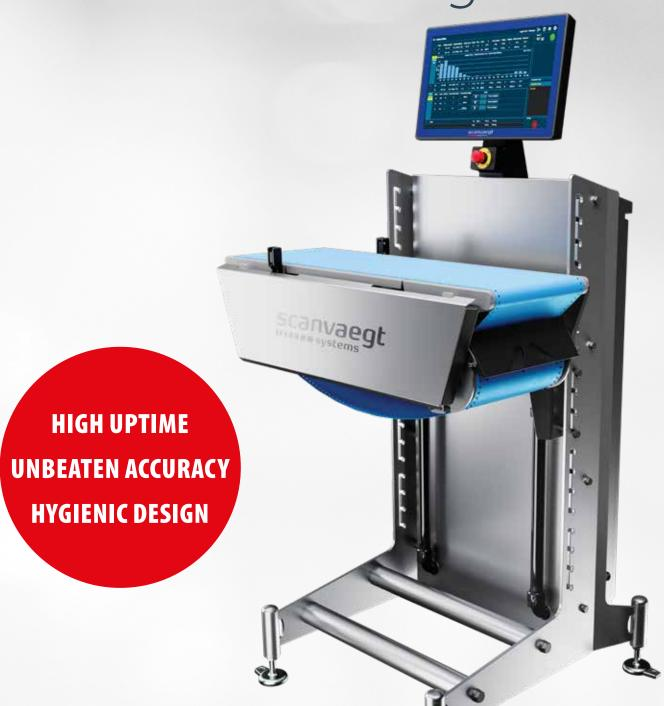
The Scanvaegt SB520 ScanBatcher is the next generation dynamic weighing machine, which represents a fast, cost-effective and sturdy solution for various applications e.g. minimum batching, tolerance batching and sizing.
