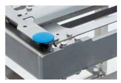
Heavy rubber shock-absorber under plate
