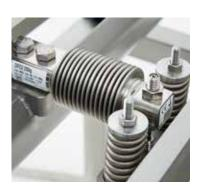
Hermetically sealed, stainless steel load cell
